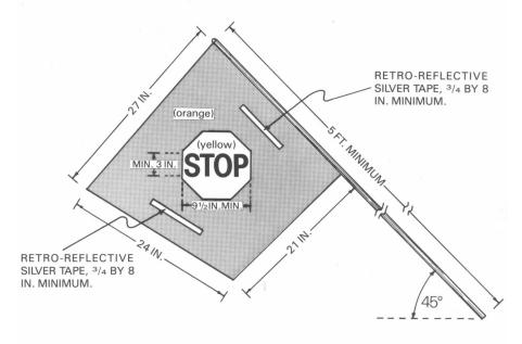
Held at a 45 degree angle, stop sign is parallel to ground.
