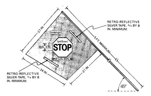
Held at a 45 degree angle, stop sign is parallel to ground.
