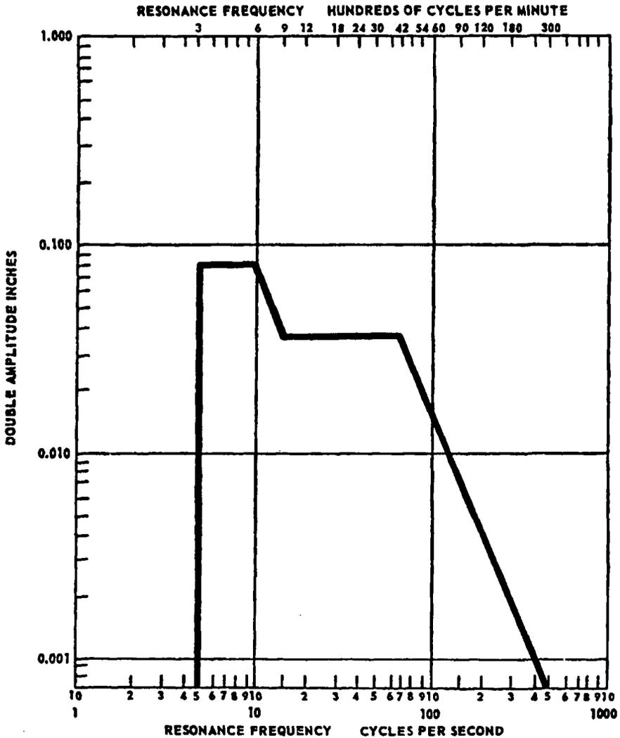
FIGURE 1: AMPLITUDE OF VIBRATION AT RESONANCE FREQUENCY
