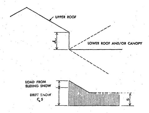
DESIGN LOWER ROOF OR CANOPY FOR LOADS ACCORDING TO FIGURE II + 50% of DESIGN LOAD FROM UPPER. THE DISTRIBUTION SHOULD BE MADE DEPENDING ON THE RELATIVE SIZES, SLOPES AND POSITIONS OF THE TWO ROOFS.
