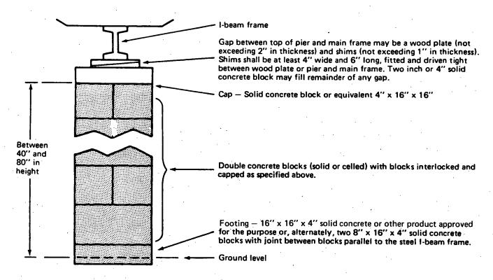
Footing placed on firm undisturbed soil or on controlled fill free of grass and organic materials compacted to a minimum load-bearing capacity of 2000 PSF.
